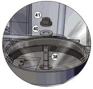
Inside Hopper: Spindle (Item 38) comes up through the base plate weldment. Washer (Item 40) is held down to base plate by Grommet (Item 41), to keep material from falling out around spindle.
